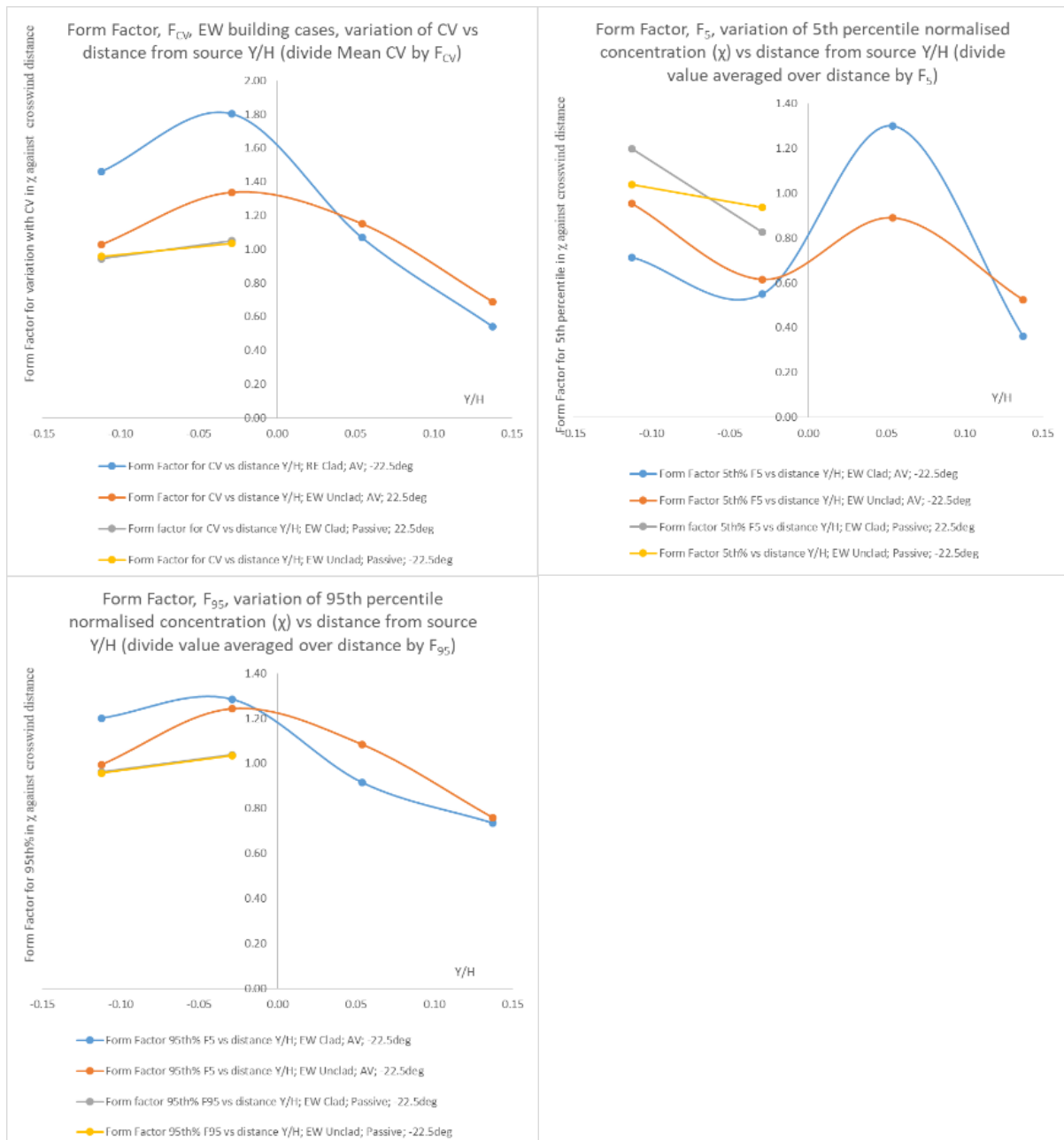
Figure 15.4.12(a/b/c): EW passive and active vertical results – crosswind form factor F_y vs Y/H : fixed angle of incidence -22.5°; fixed distance from the source X/H=0.67 ; active vertical (AV) Z_{RH}=255\text{mm} ; passive Z_{RH}=245\text{mm} ; (a) CV (top left); (b) 5 th percentile (top right); (c) 95 th percentile (below)
