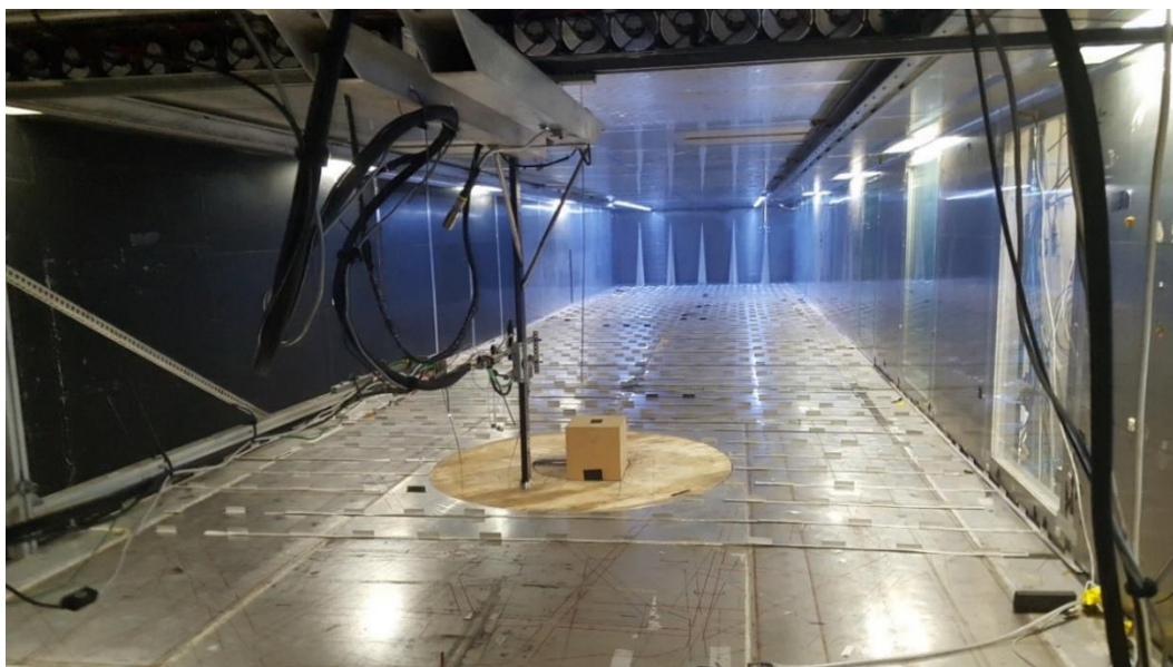
Figure 3.2: Interior of the wind tunnel looking upstream with the cube model in place
