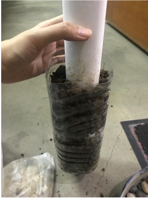
Figure 14 Fill outer core with soil.
