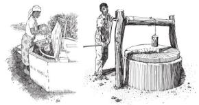
An <u>unprotected dug well</u> is a dug well for which one or both of the following are true: (1) the well is not protected from run-off water; (2) the well is not protected from bird droppings and animals. If at least one of these conditions is true, the well is unprotected.
