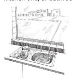
• <u>Piped into compound, yard or plot</u>, also called a yard connection, is defined as a piped water connection to a tap placed in the compound, yard or plot outside the house.
