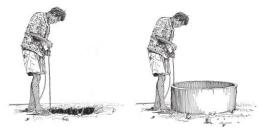
A <u>protected spring</u> is a spring that is free from run-off and from bird droppings and animals. A spring is typically protected by a 'spring box' that is constructed of brick, masonry or concrete and is built around the spring so that water flows directly out of the box into a pipe without being exposed to outside pollution.
