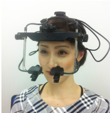
Example of an eye tracking system used in our experiments (EyeLink II, SR research; http://sr-research.jp/products/images/eyelink2_head.jpg )
