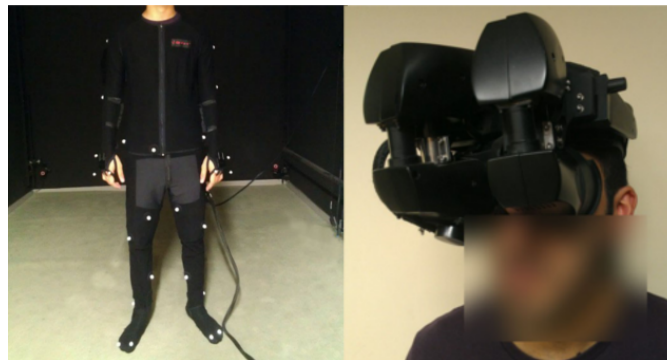
Figure 1: Full-body motion capture suit (left) and HMD (right).
