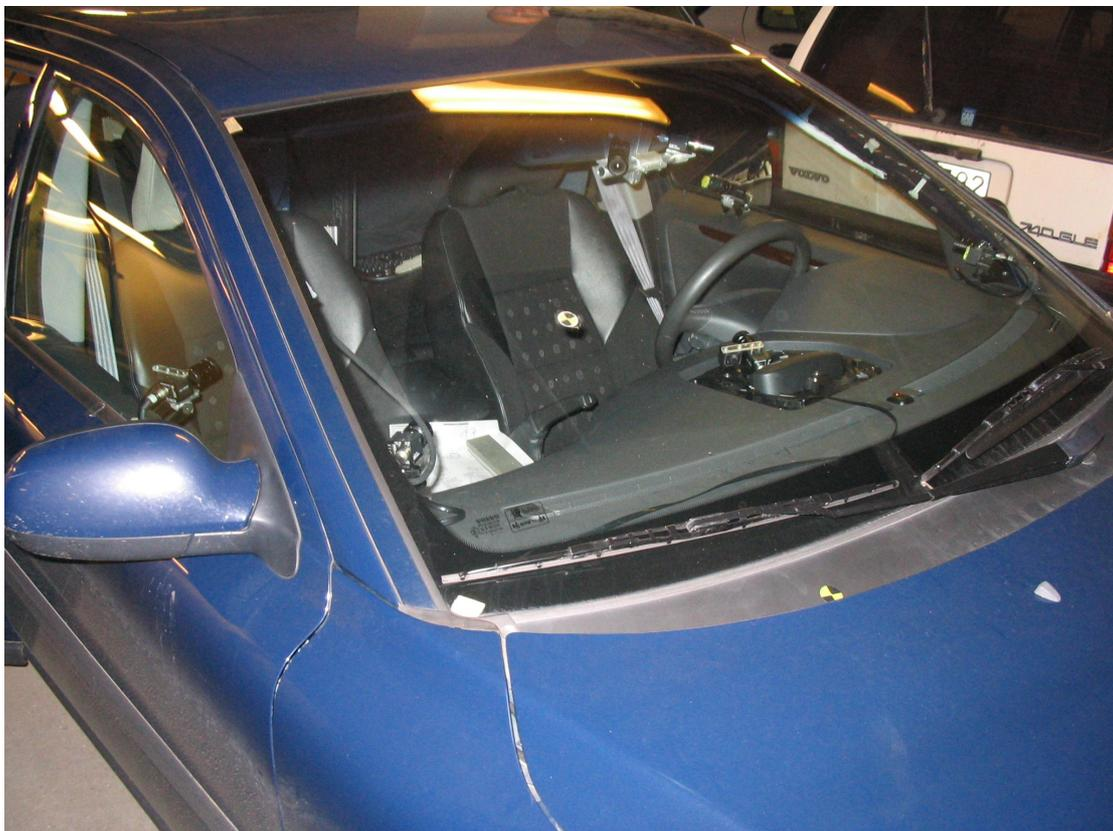
*FIGURE 2. A four camera system mounted in an instrumented car.*
